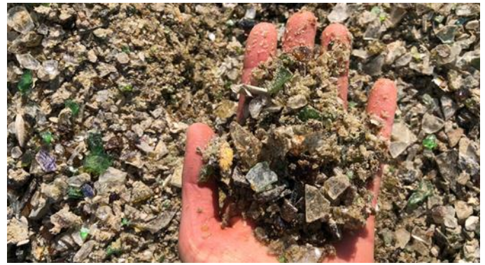
PGA crushed to 1" or less (NHDES specification)
